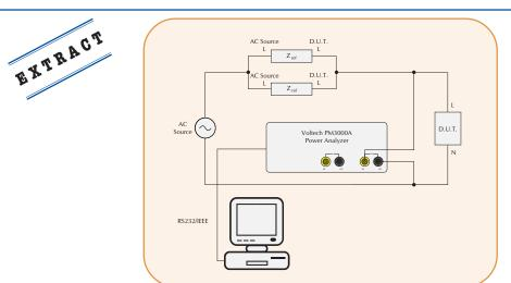
The impedance is defined to be a complex one, consisting of both resistive and inductive elements. The 61000-3-3 impedance is called  $\rm Z_{ref}$  in 61000-3-11 and consists of 0.40 ohms resistive in series with 0.25 ohms inductive at 50Hz.
