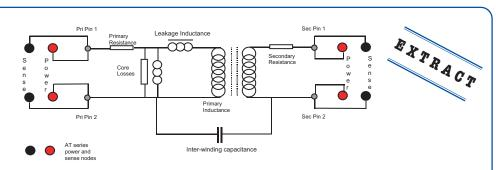
From the schematic in figure 1, it can be seen that even the most simple of transformers includes quite a complex combination of resistive and reactive components. In order to establish with confidence that a transformer has been manufactured correctly, it is necessary to execute a range of tests that combine to provide an assurance that the materials used and manufacturing process executed results in transformers that meet the design specification.
